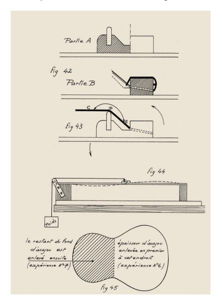
Part A will precisely define the end of the vibrating string length, and the height of the saddle will insert itself under the string, raising it upwards, letting the string tension apply pressure and torsion when combining parts A and B.
