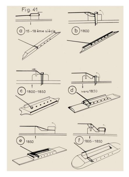
The bridge transmits string vibrations to the soundboard. It is the final component to be glued during the construction process. For over one hundred years, its shape and structure have been refined to suit guitars played with fingers.
