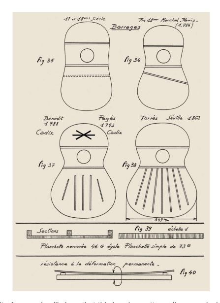
A little bit of research will show that this bracing pattern allows equivalent longitudinal rigidity and solidity while maximising transversal flexibility with less thickness. All that is required is to glue three braces on a softwood board 40 cm long and 2.6 mm thick (fig. 39), and it will become apparent that a board 5.2 millimetres thick is required to provide the same amount of flexibility, the same resistance, and will weigh 73 grams instead of 46 grams.
