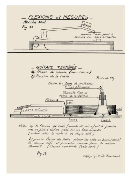
10) Soundboard flexibility – strings tuned to pitch – strings slack. Without changing the guitar's position on the apparatus, following the previous measurement, move on to the measurement concerning the soundboard's flexibility once the guitar is complete. The 8 kg weight is inserted between the transverse slats (as described above) and applies weight to the bridge, positioned temporarily before varnishing.
